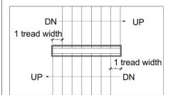
AS1428.1 at the CC stage of works. **Note:** For stairways with 90° to 180° turns at landings, in order for the handrails to comply with the consistent height requirement, the risers have to be offset at the mid-landings OR provided with a 300mm handrail extension, so that no vertical sections are created in the handrails. This applies to both non-fire-isolated and fire-isolated stairways.
