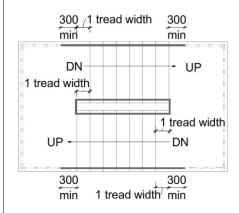
**Note:** In some cases, the stairway from the basement to the ground floor level is considered to be non-fire-isolated, in which case full compliance will be required as per AS1428.1-2009. Verify with the BCA consultant.
