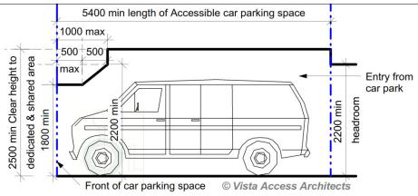
Head heights for both dedicated accessible parking space and the shared zone to be as shown above. No beams, pipes, sprinklers or any other encroachments are persmissible for the entire 5.4M width of the dedicated and shared zone as per Section shown above.
