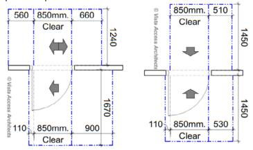
Note that the circulation spaces (other than doorway threshold ramp) to have a maximum floor grade of 1:40. Where there is a level difference at the door threshold, the maximum level difference can be 35mm if provided with a 1:8 doorway threshold ramp. This is achievable and the door selections are to be verified at CC stage of works.
